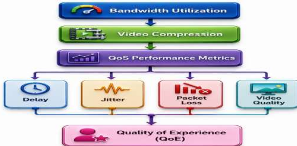
Figure 2: Relationship between bandwidth optimization, QoS parameters, and QoE in live video streaming.
