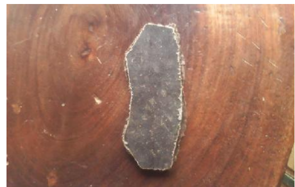
Plate 3.5: 25 wt% Resin Water Melon Peels Brake Pad produced
